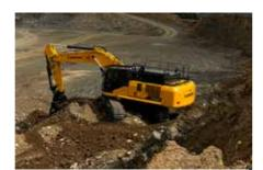
**ENGINE:** Cummins **NET POWER:** 260 hp @ 2,000 RPM 51,000 kg **BASE OP WEIGHT:**
